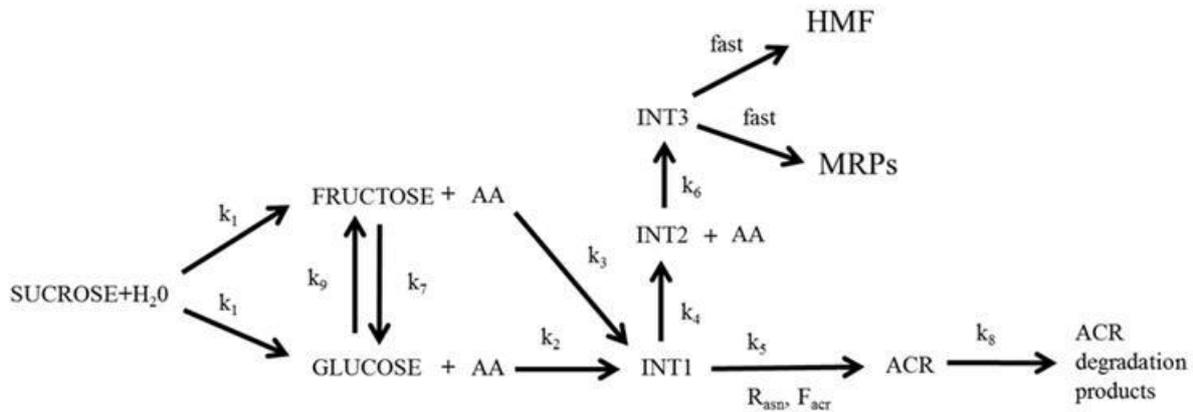
Figure 27. Simplified kinetic scheme selected by model discrimination analysis
